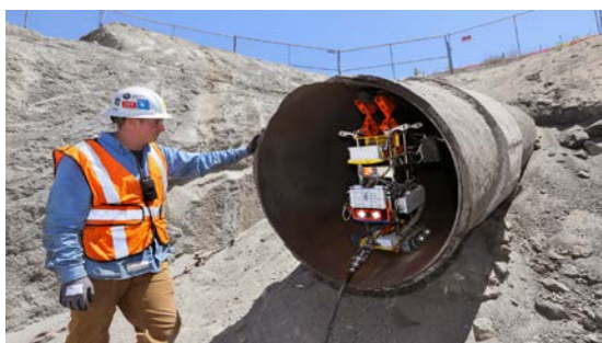
Deployment of a robotic condition assessment tool on the First Aqueduct
