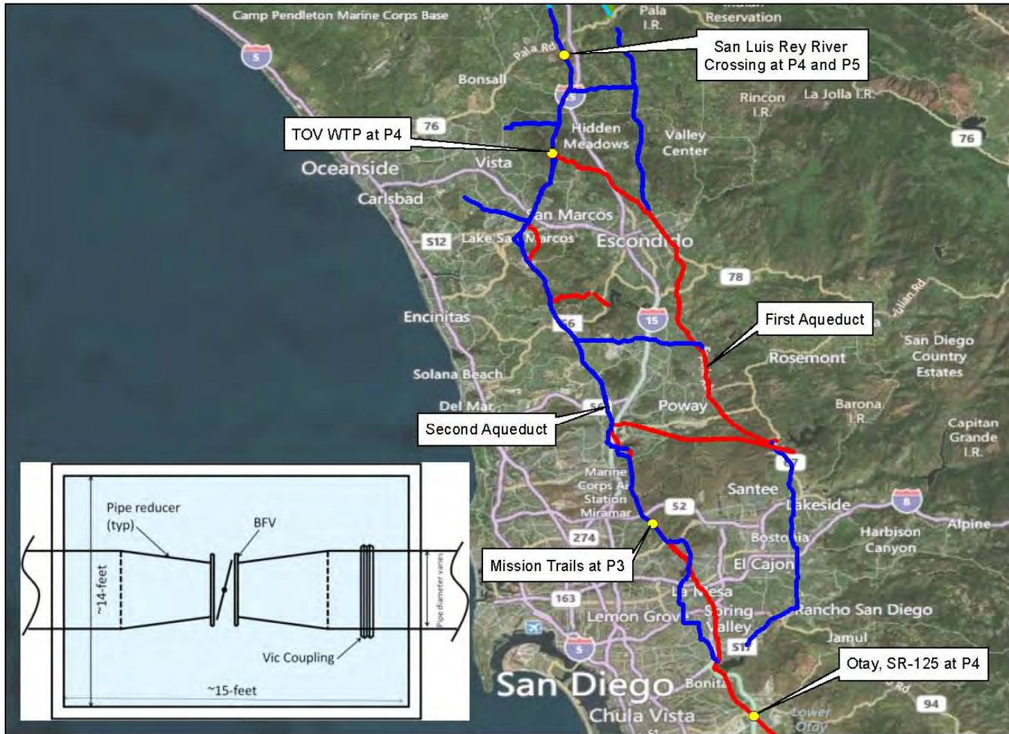
San Diego County Water Authority 2013 Regional Water Facilities Master Plan Update Figure 7-9 System Isolation Valves
