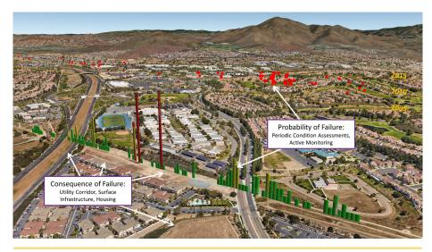
Probability of Failure and Consequence of Failure monitoring.
